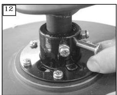
Align hole in downrod with hole in yoke and install cross pin.
